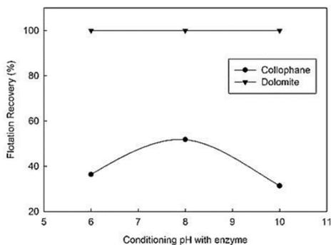
Fig. 3. Effect of conditioning pH, with enzyme, on floatability of collophane and dolomite single minerals in presence of cellulase using  $2 \cdot 10^{-4}$  mol/dm<sup>3</sup> oleic acid
