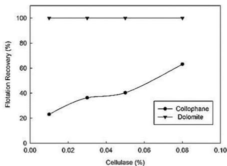
Fig. 2. Effect of cellulase concentration on floatability of collophane and dolomite single minerals using  $2 \cdot 10^{-4}$  mol/dm<sup>3</sup> oleic acid
