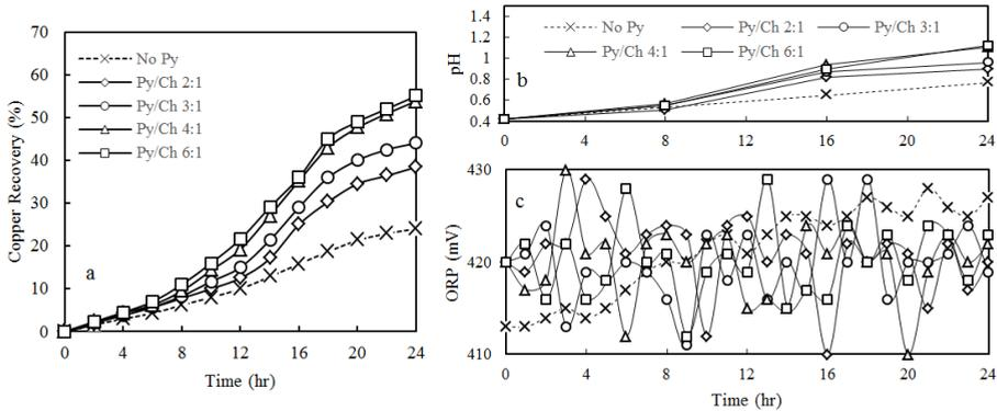
Fig. 1. (a) Copper recovery for different Py/Ch mass ratios, (b) pH, and (c) ORP values during leaching experiments. Conditions: temperature of 80 °C, 0.11 mol/dm<sup>3</sup> total iron, 0.4 mol/dm<sup>3</sup> sulfuric acid (initial pH of 0.42), potential range of 410-430 mV [Pt vs. Ag/AgCl], 850 rpm stirring speed
