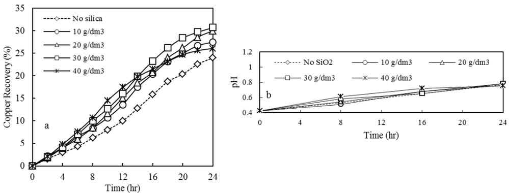
Fig. 5. (a) Copper recovery for different concentrations of silica, (b) pH values during leaching experiments. Conditions: temperature of 80 °C, 0.11 mol/dm<sup>3</sup> total iron, 0.4 mol/dm<sup>3</sup> sulfuric acid (initial pH of 0.42), potential range of 410–430 mV [Pt vs. Ag/AgCl], 700 rpm stirring speed
