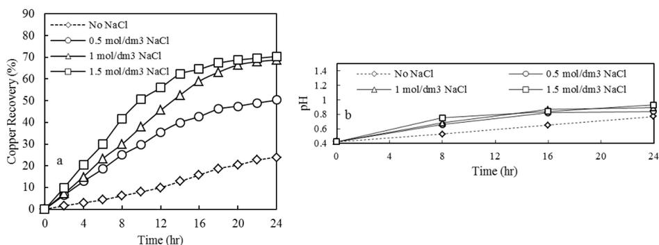
Fig. 2. (a) Copper recovery for different sodium chloride concentrations, (b) pH values during leaching experiments. Conditions: temperature of 80 °C, 0.11 mol/dm<sup>3</sup> total iron, 0.4 mol/dm<sup>3</sup> sulfuric acid (initial pH of 0.42), potential range of 410-430 mV [Pt vs. Ag/AgCl], 850 rpm stirring speed
