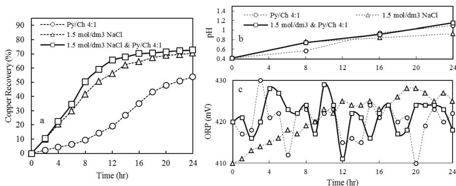
Fig. 3. (a) Copper recovery in the presence of pyrite, sodium chloride and both, (b) pH and (c) ORP values during leaching experiments. Conditions: temperature of 80 °C, 0.11 mol/dm<sup>3</sup> total iron, 0.4 mol/dm<sup>3</sup> sulfuric acid (initial pH of 0.42), potential range of 410-430 mV [Pt vs. Ag/AgCl], 850 rpm stirring speed
