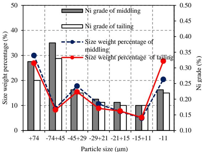
Fig. 3. Size analysis of circulating middling and tailing
