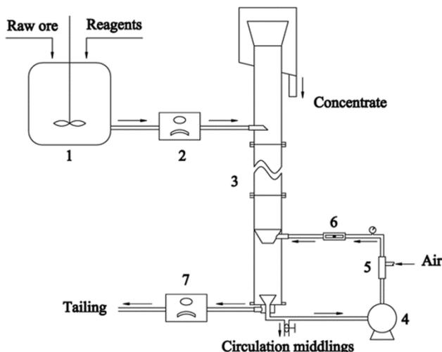
Fig. 1. Schematic illustration of the lab-scale cyclonic flotation column system.
