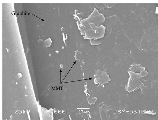
Fig. 5. SEM of graphite coated with colloidal MMT
