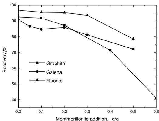
Fig. 4. Effect of various MMT additions in the slurry on the recovery of three minerals
