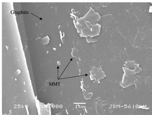
Fig. 5. SEM of graphite coated with colloidal MMT
