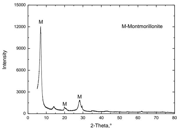
Fig. 1. XRD trace of the colloidal MMT
