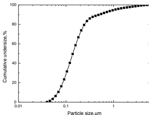
Fig. 3. Particle size distribution of colloidal MMT samples
