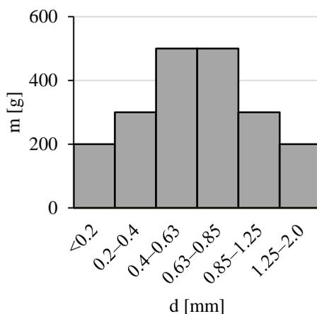
Fig. 3. A particulate composition for mixtures (the rotary and drum screen with a cone-shaped sieve):
