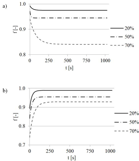
Fig. 8. Impact of the amount of hard-to-screen grains in the feed on screen blocking coefficient (a laboratory vibrator and control sieves): a) when  $f_0 > f_\infty$  (spherical grains,  $l = 0.63$  mm,  $K = 3.5$ ), b) when  $f_0 < f_\infty$  (irregular grains,  $l = 0.63$  mm,  $K = 35$ )
