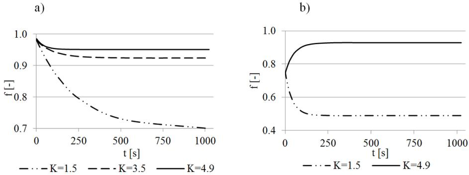
Fig. 9. Impact of the value of the vibrating device toss indicator on sieve holes blocking (laboratory vibrator and control sieves), a) spherical grains,  $l = 1$  mm, b) irregular grains,  $l = 0.5$  mm
