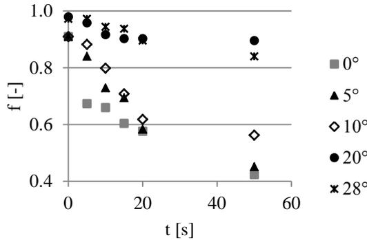
Fig. 10. Impact of the angle of inclination of a drum in a rotary and drum device on screen blocking coefficient (irregular grains,  $l = 0.6$  3mm, drum (sieve) rotational speed 0.7 rpm, efficiency  $Q = 135$  kg/h)
