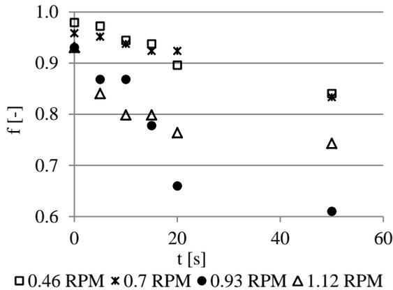
Fig. 11. Impact of the disk rotational speed in a rotary and drum device on the screen blocking coefficient (irregular grains,  $l = 0.63$  mm, sieve inclination angle  $20^\circ$ , efficiency  $Q = 182$  kg/h)
