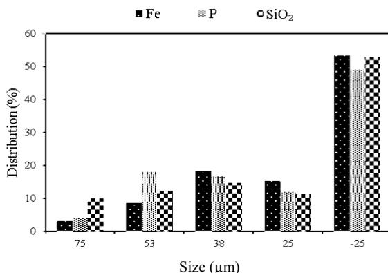
Fig. 3. Distribution of iron, phosphorus, and silica contents of Chadon-malu final magnetic concentrate as a function of particle size
