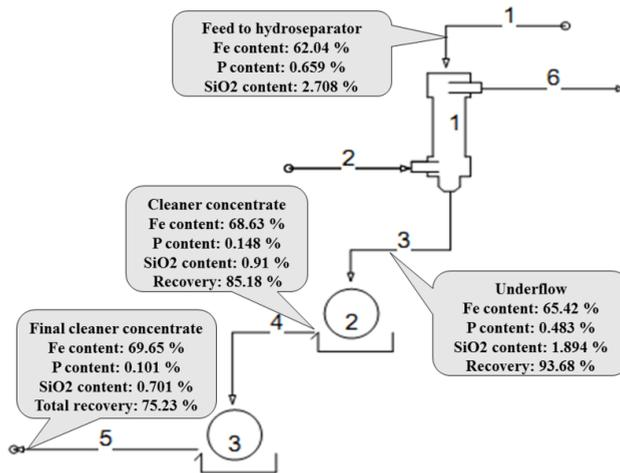
Fig. 10. Combining hydroseparator with low intensity magnetic separator
