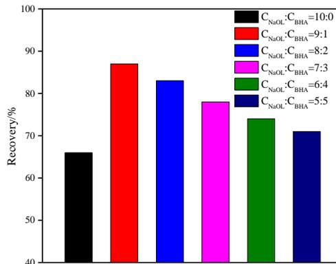
Fig. 4. Recovery of wolframite at various ratios of NaOL and BHA
