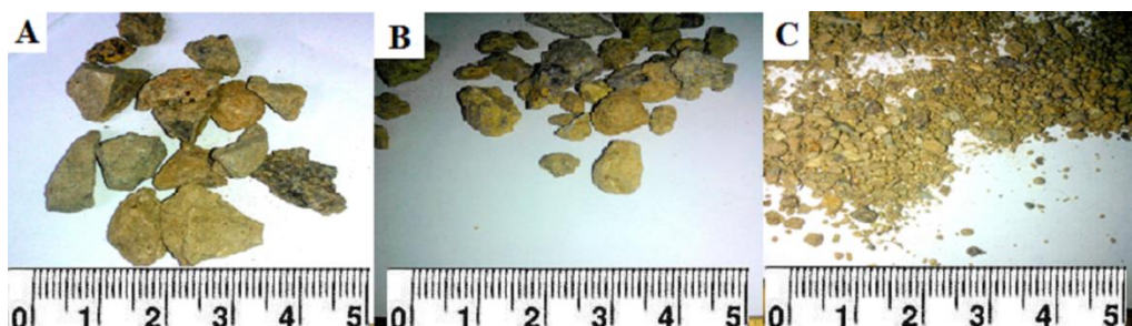
Fig. 1. Representative ore fractions before leaching. (A) 10–20 mm, (B) 2.5–10 mm, (C) 0.5–2.5 mm
