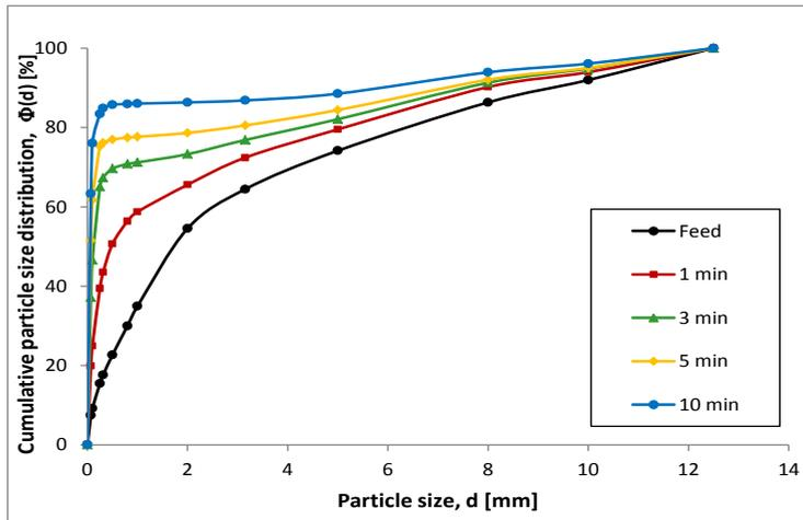
Fig. 4. Grinding kinetics for feed material from Polkowice
