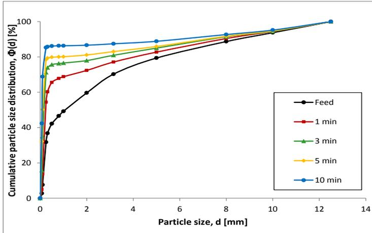
Fig. 3. Grinding kinetics for feed material from Rudna
