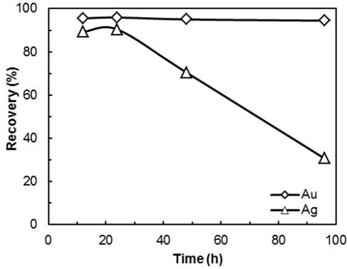
Fig. 2. Effect of leaching time on gold and silver recoveries (1  $\text{g}/\text{dm}^3$  NaCN concentration, 10% solids ratio, -100  $\mu\text{m}$  particle size, and 450 rpm stirring speed at room temperature)
