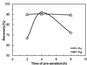
Fig. 6. Effect of time of pre-aeration (40% solids ratio, 4 g/dm<sup>3</sup> NaCN concentration, 12 h cyanidation time after pre-aeration time of 2, 4, and 8 h, -74 µm particle size, and 450 rpm stirring speed at room temperature)
