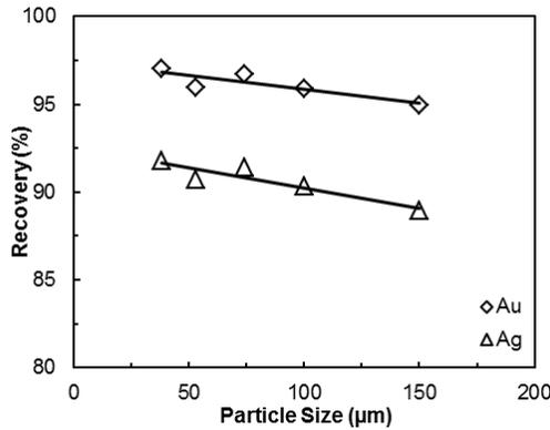
Fig. 4. Effect of particle size on gold and silver recoveries (10% solids ratio, 1  $\text{g}/\text{dm}^3$  NaCN concentration, 24 h cyanidation time, and 450 rpm stirring speed at room temperature)
