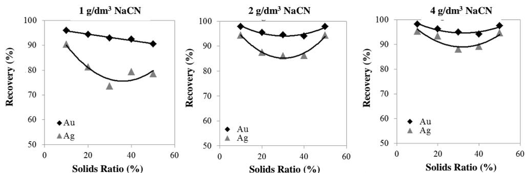
Fig. 5. Effect of solids ratio in the presence of 1-2-4  $\text{g/dm}^3$  NaCN (24 h cyanidation time,  $-74 \mu\text{m}$  particle size, and 450 rpm stirring speed at room temperature)
