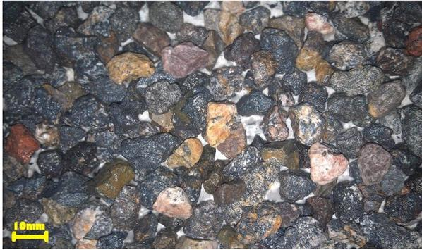
Fig. 4. Initial iron-phosphate ore particles shape
