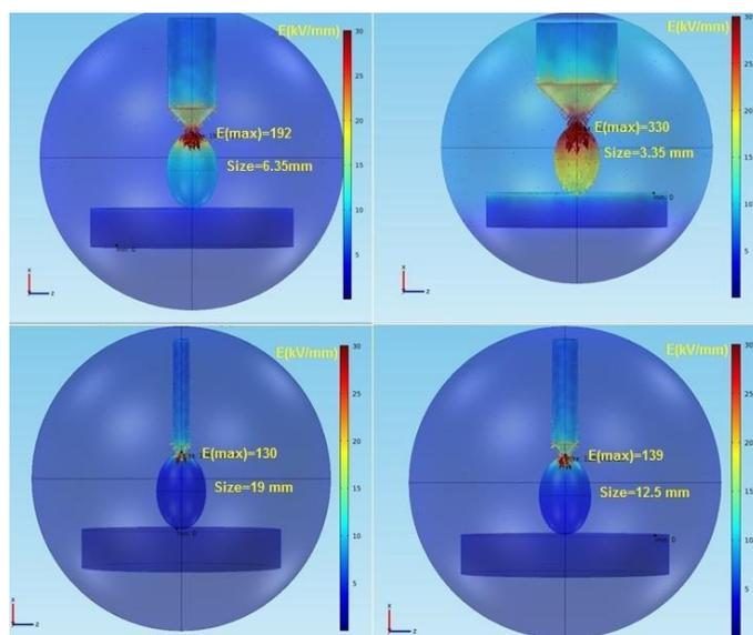
Fig. 11. Numerical simulation of the effect of feed size on electrical field intensity and distribution (front view)
