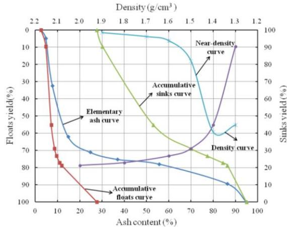
Fig. 1. Washability curves of 6-1mm fine coal sample
