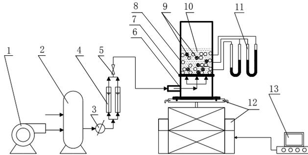
Fig. 2. Experimental apparatus of vibration fluidized bed
