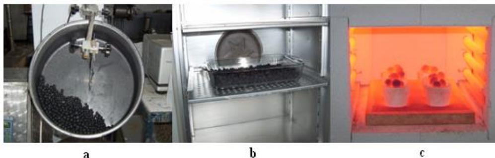
Fig. 2. (a) Green, (b) dry, (c) fired pellets
