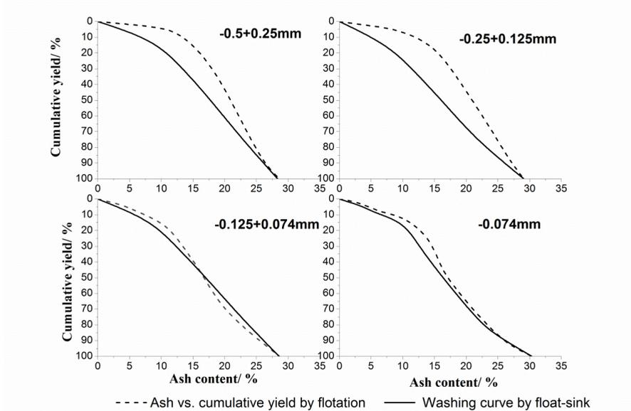
Fig. 5. Cumulative yield vs. ash of ground products separated by float-sink and progressive release flotation
