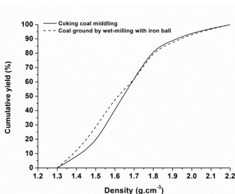
Fig. 4. Cumulative yield vs. density of coking coal middlings and ground products
