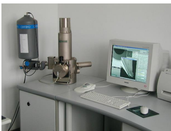
Fig. 2. Tescan Vega 5135 MM scanning electron microscope
