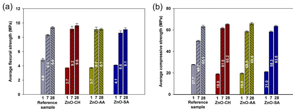
Fig. 4. Average flexural (a) and compressive (b) strength of cement mortars after 1, 7 and 28 days maturation
