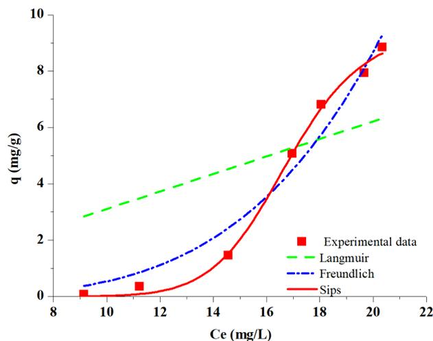
Fig. 2. Non-linear fitting of tannic acid adsorption onto fluorite
