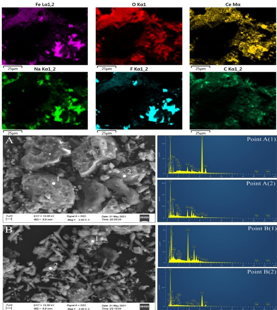
Fig. 12. SEM-EDS results for solid fluorine minerals
