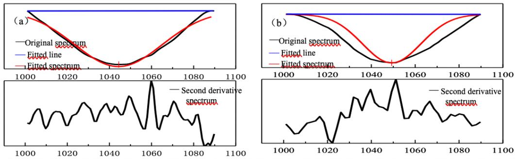
Fig. 6. Fitting spectra and second derivative spectra of fixed fluorine minerals in 1089.7-1001  $\text{cm}^{-1}$  under conventional and microwave roasting conditions (a. conventional roasting; b. microwave roasting method)
