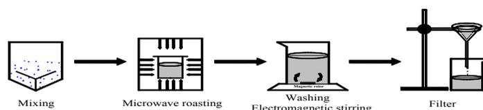
Fig. 2. Schematic diagram of experimental process and equipment
