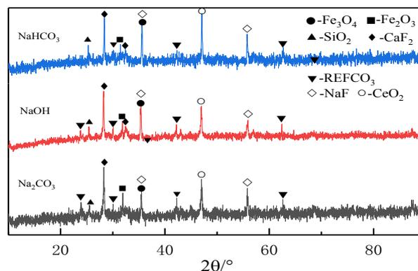
Fig. 7. Comparison of XRD patterns of Bayan Obo rare earth ore and ore roasted with different sodium fluoride fixer
