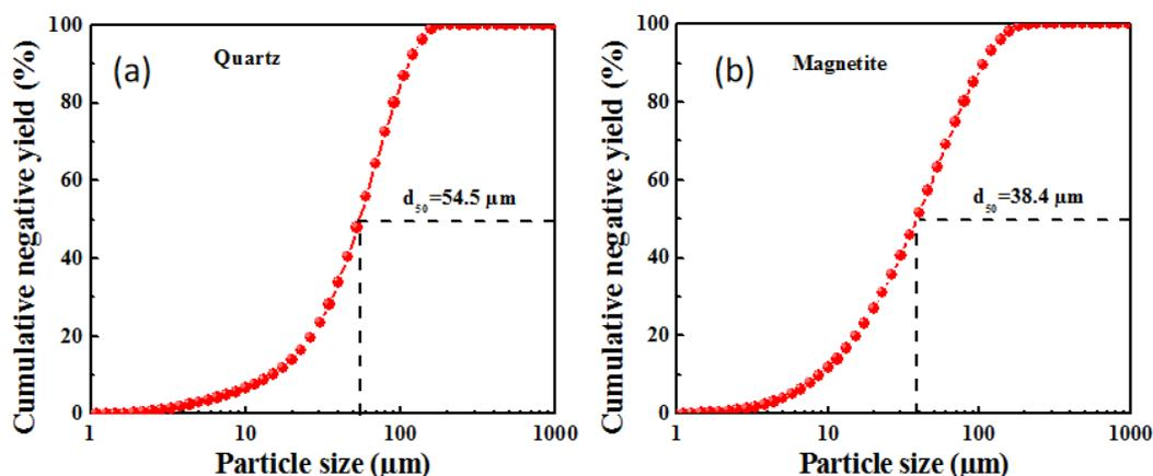
Fig. 1. Particle size distribution and cumulative distribution curve of quartz (a) and magnetite (b)
