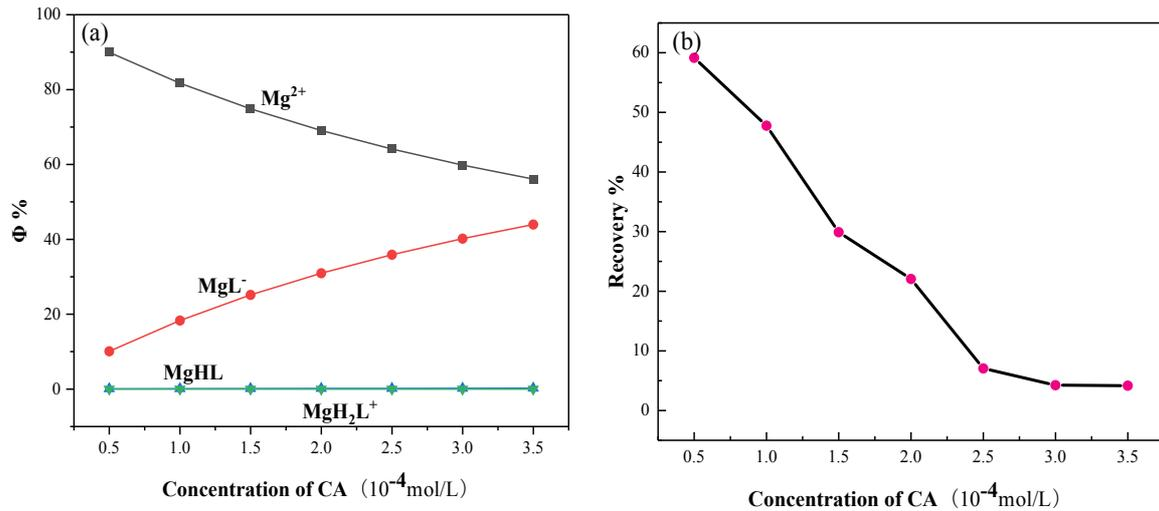
Fig. 11 (a). Distribution of CA and  $Mg^{2+}$  product components; (b). Effect of CA concentration on the flotation
