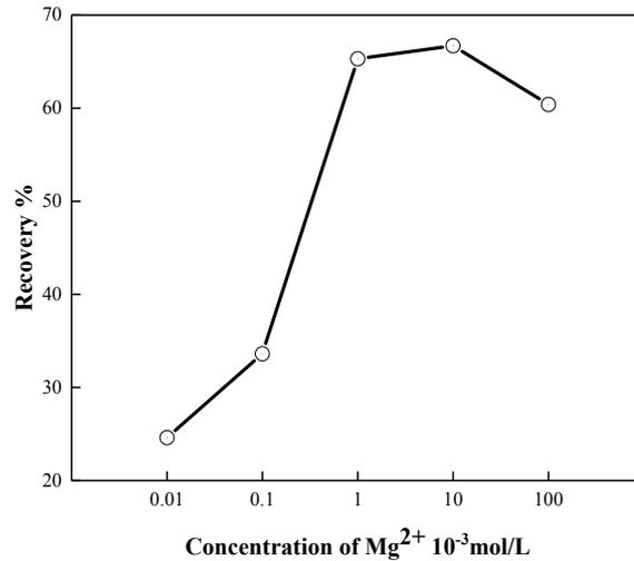
Fig. 3. Effect of  $Mg^{2+}$  concentration on flotation
