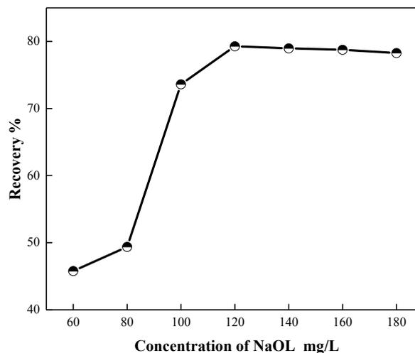
Fig. 4. Effect of Na-OI concentration on the flotation
