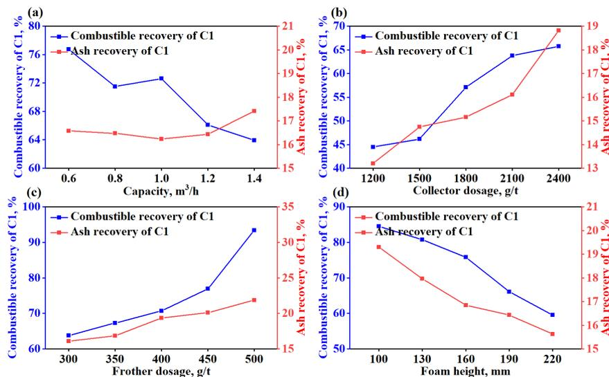
Fig. 3. Combustible matter recovery and ash content of C1 with various flotation parameters: (a) capacity, (b) collector dosage, (c) frother dosage, and (d) foam height
