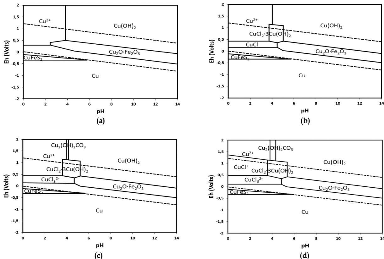
Fig. S6. Pourbaix Diagrams for  $\text{CuFeS}_2$  at 25 °C and 0.07 m of Cu, ions effect (Br<sup>-</sup>,  $\text{CO}_3^{2-}$ ,  $\text{Cl}^-$ )
