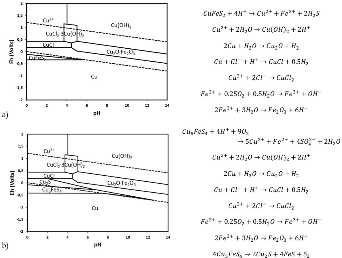
Fig. 2. Pourbaix Diagrams for seawater 35 % at 298 K and 0.07 m of Cu, ions effect (Br-,  $\text{CO}_3^{2-}$ , Cl-). a) Solid species  $\text{CuFeS}_2$ , b) Solid Species  $\text{Cu}_5\text{FeS}_4$
