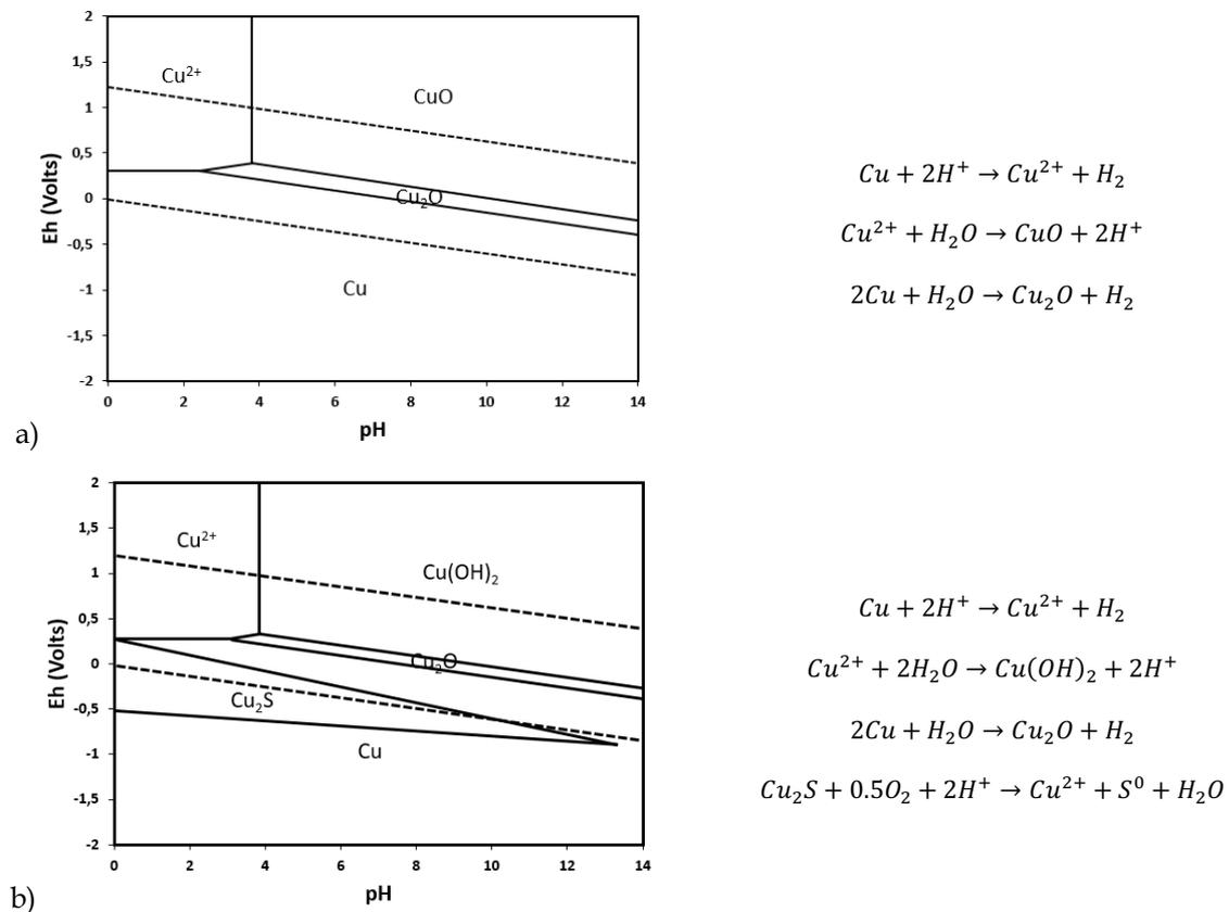
Fig. 1. Pourbaix Diagrams for pure water 0 ‰ at 298 K and 0.07 m of Cu. a) Solid species CuO, b) Solid species Cu<sub>2</sub>S
