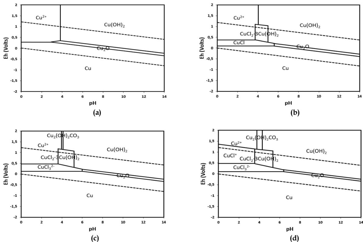
Fig. S1. Pourbaix Diagrams for  $\text{Cu}_2\text{O}$  at 25 °C and 0.07 m of Cu, ions effect ( $\text{Br}^-$ ,  $\text{CO}_3^{2-}$ ,  $\text{Cl}^-$ )
