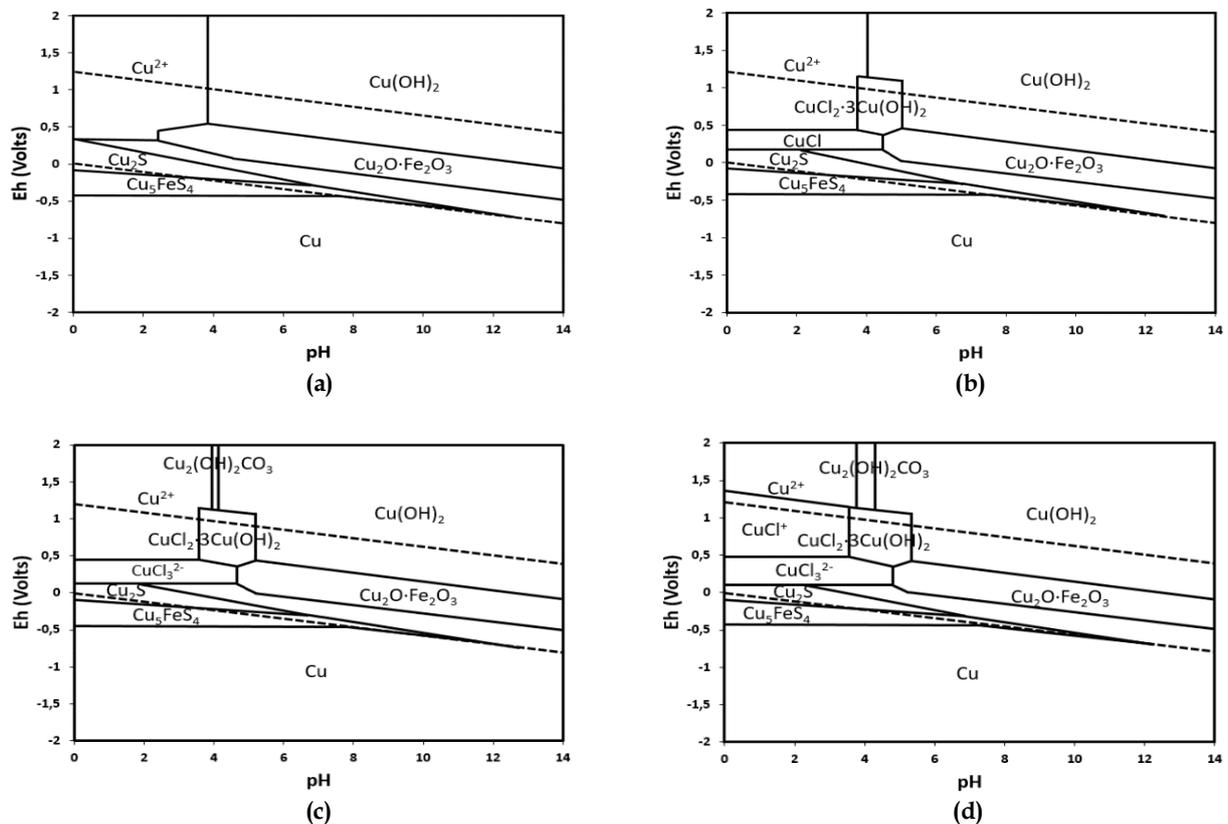
Fig. S5. Pourbaix Diagrams for  $\text{Cu}_5\text{FeS}_4$  at 25 °C and 0.07 m of Cu, ions effect ( $\text{Br}^-$ ,  $\text{CO}_3^{2-}$ ,  $\text{Cl}^-$ )
