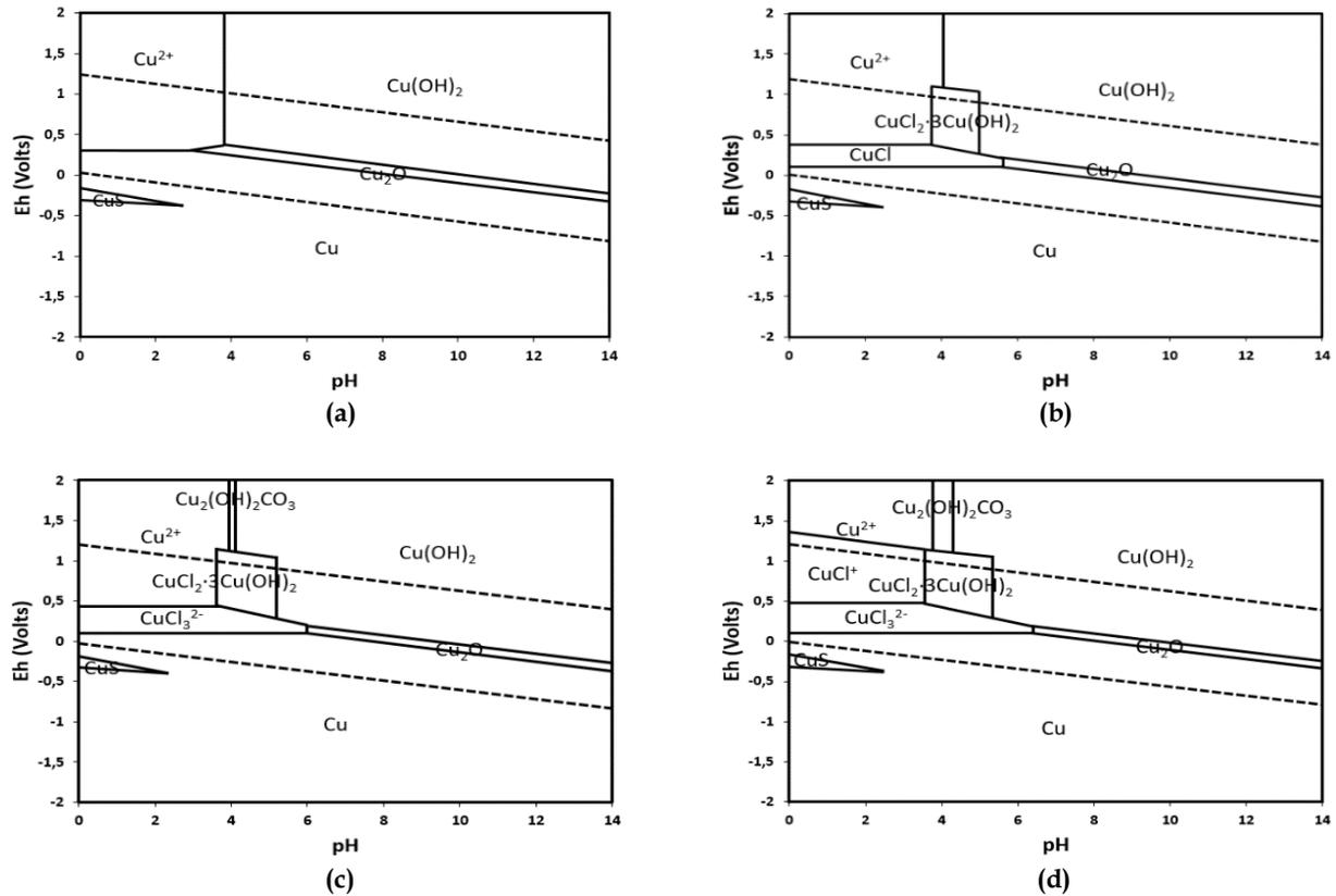
Fig. S4. Pourbaix Diagrams for CuS at 25 °C and 0.07 m of Cu, ions effect ( $\text{Br}^-$ ,  $\text{CO}_3^{2-}$ ,  $\text{Cl}^-$ )
