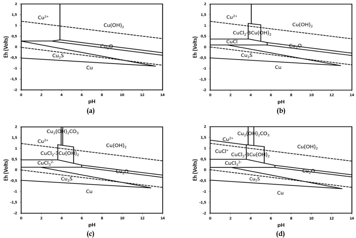
Fig. S3. Pourbaix Diagrams for Cu<sub>2</sub>S at 25 °C and 0.07 m of Cu, ions effect (Br<sup>-</sup>, CO<sub>3</sub><sup>2-</sup>, Cl<sup>-</sup>)
