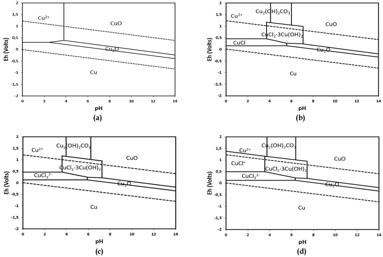
Fig. S2. Pourbaix Diagrams for CuO at 25 °C and 0.07 m of Cu, ions effect (Br<sup>-</sup>, CO<sub>3</sub><sup>2-</sup>, Cl<sup>-</sup>)
