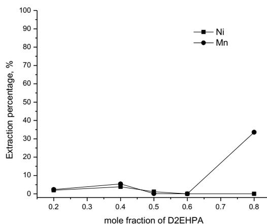
Fig. 6. Effect of mole fraction of D2EHPA in the mixture on the extraction of Mn(II) and Ni(II) from solution with pH 2.95. (The concentration of D2EHPA and Alamine 336 in the mixture was fixed at 0.5 M and 10% decanol was present as a modifier)
