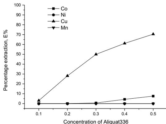
Fig. 1. Effect of Aliquat 336 concentration on the extraction of Cu(II) from 3 M HCl solution
