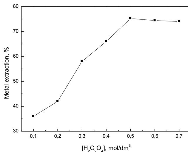
Fig. 4. Effect of acid concentration on the leaching efficiency of Al(III)
