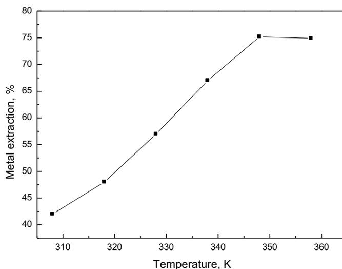
Fig. 2. Effect of temperature on the leaching efficiency of Al(III)
