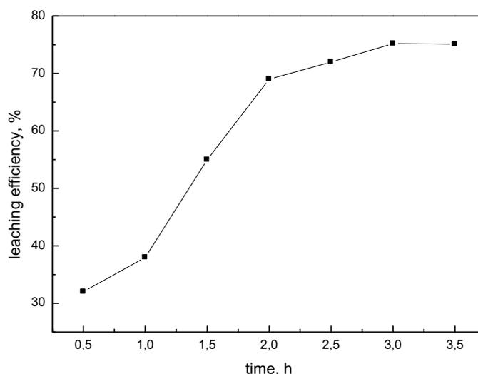
Fig. 5. Effect of contact time on the leaching efficiency of Al(III)
