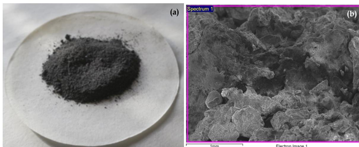
Fig. 1. Milled aluminum dross (a) SEM micrograph of the aluminum dross (b)
