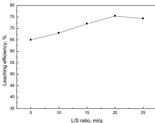
Fig. 3. Effect of liquid to solid ratio (L/S)
