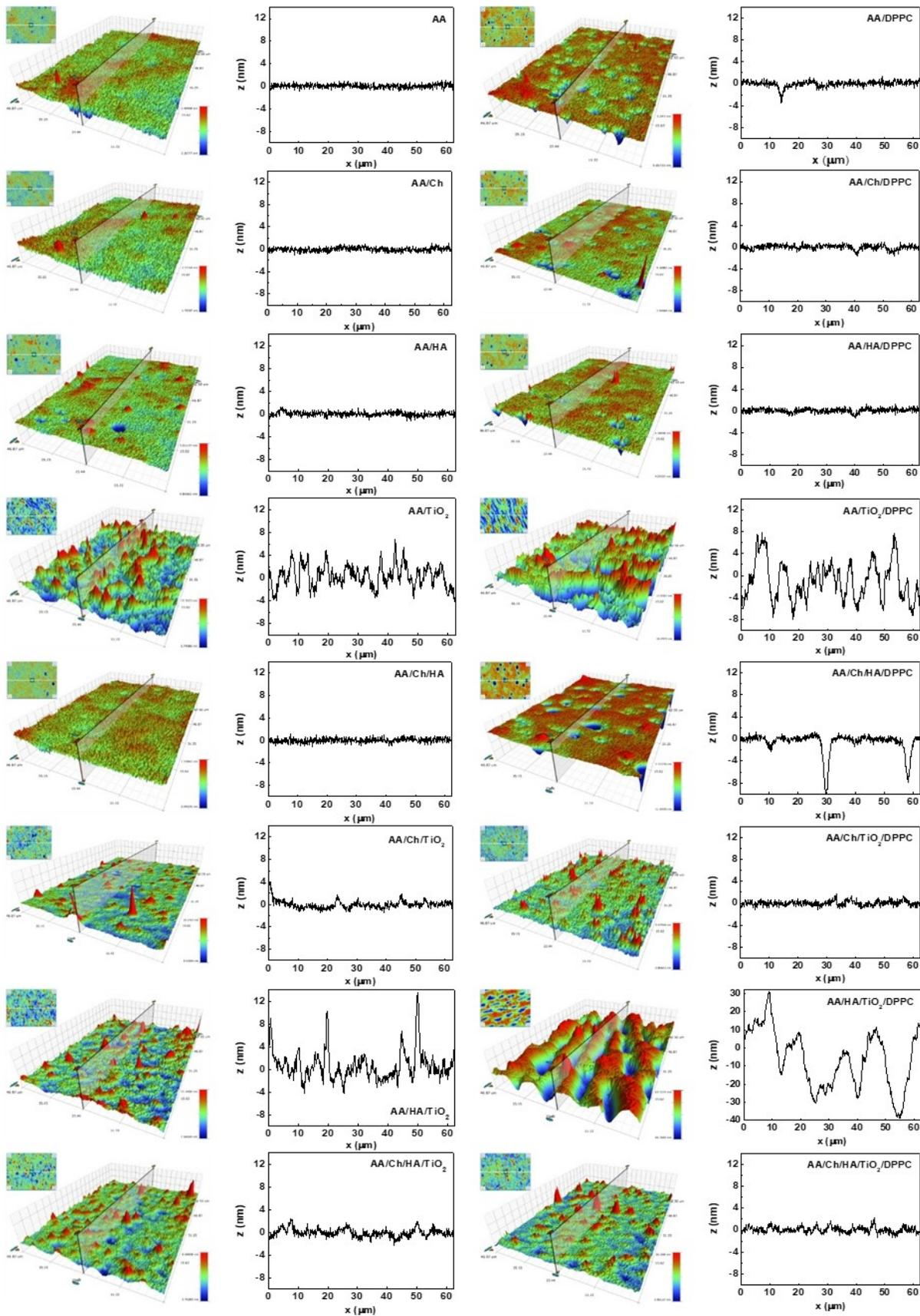
Fig. 1. Profilometric 2D and 3D images with the cross-section (profiles) along the sheet for the air plasma activated glass plates covered with the films of AA, AA/Ch, AA/HA, AA/TiO<sub>2</sub>, AA/Ch/HA, AA/Ch/TiO<sub>2</sub>, AA/HA/TiO<sub>2</sub>, AA/Ch/HA/TiO<sub>2</sub>, with or without the DPPC monolayer (the image size 47 μm x 62 μm)
