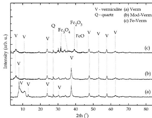
Fig. 3. X-ray diffraction patterns of vermiculite and its modified forms: natural vermiculite (a), acid treated and Al<sub>2</sub>O<sub>3</sub>-pillared vermiculite (b), Fe-vermiculite (c)
