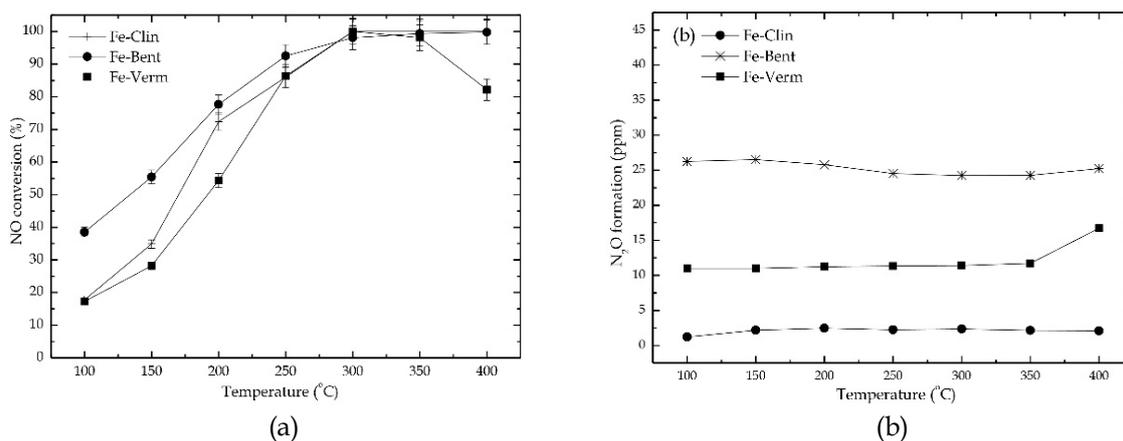
Fig. 6. NH<sub>3</sub>-SCR catalytic performance of the studied samples: NO conversion (a), N<sub>2</sub>O formation (b) (experimental conditions: [NO] = 800 ppm, [NH<sub>3</sub>] = 800 ppm, [O<sub>2</sub>] = 3.5 vol.%, balance He, total flow of the gas mixture: 100 cm<sup>3</sup>·min<sup>-1</sup>, mass of the catalyst: 200 mg)
