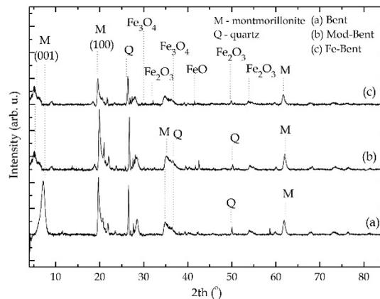
Fig. 2. X-ray diffraction patterns of parent bentonite and its modified forms: natural bentonite (a), acid treated and Al<sub>2</sub>O<sub>3</sub>-pillared bentonite (b), Fe-bentonite (c)
