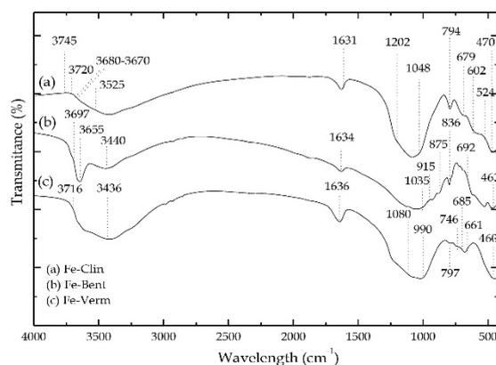
Fig. 4. FT-IR spectra of Fe-Clin (a), Fe-Bent (b), Fe-Verm (c) in a region of  $4000$  to  $450\text{ cm}^{-1}$
