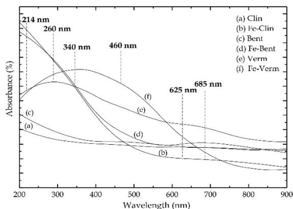
Fig. 5. UV-Vis spectra of Clin (a), Fe-Clin (b), Bent (c), Fe-Bent (d), Verm (e), Fe-Verm (f)
