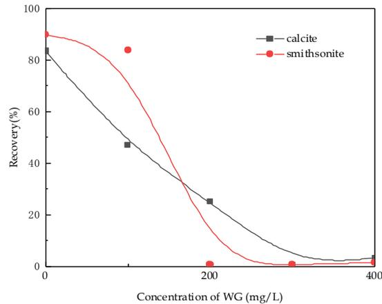
Fig. 8. Flotation results of smithsonite and calcite at pH 9 as a function of tannin concentration with  $1 \times 10^{-4}$  mol/L ODA
