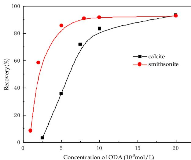
Fig. 4. Flotation results of smithsonite and calcite as a function of ODA concentration at pH 9
