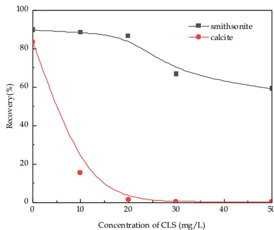
Fig. 9. Flotation results of smithsonite and calcite at pH 9 as a function of CLS concentration with  $1 \times 10^{-4}$  mol/L ODA
