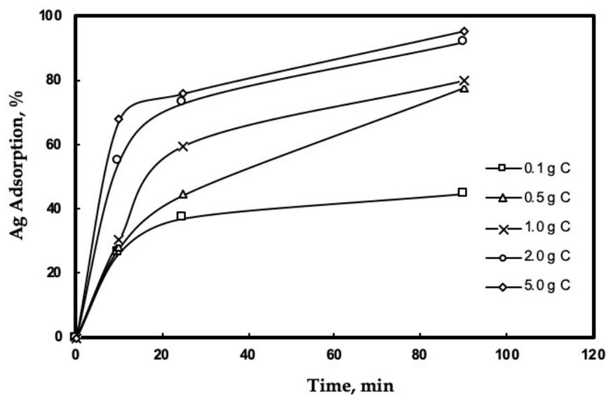
Fig. 9. Adsorption of Ag from real leach solutions initially contained 0.2 M ATS in presence of 0.01 M APS on different amounts of AC
