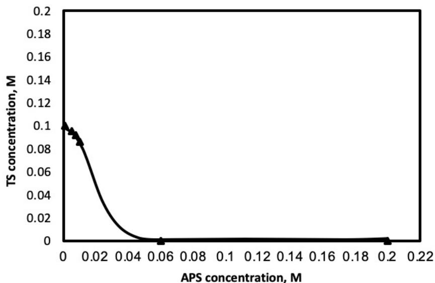
Fig. 7. Effect of initial APS concentration on free TS concentration remained in real leach solution after adsorption on AC, 90 min
