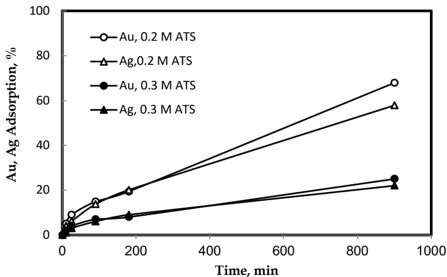
Fig. 2. Adsorption of gold and silver on AC from real leach solutions at different initial ATS concentrations
