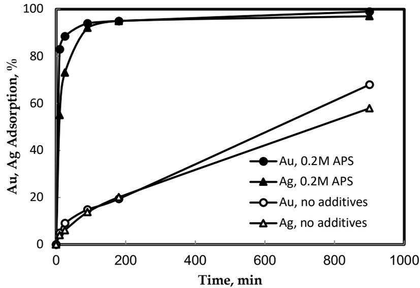
Fig. 3. Adsorption of gold and silver from real leach liquor on AC in absence and presence of 0.2 M APS
