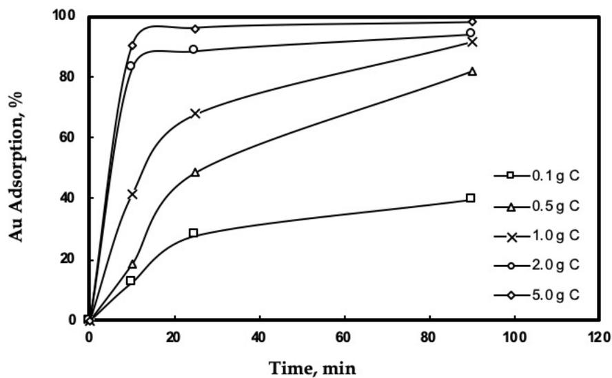
Fig. 8. Adsorption of Au from real leach solutions initially contained 0.2 M ATS in presence of 0.01M APS on different amounts of AC
