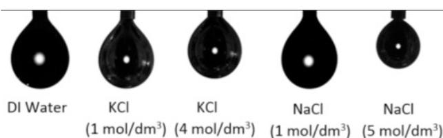
Fig. 1. Bubble images at different salt concentrations
