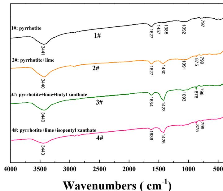
Fig. 7. IR spectra of pyrrhotite with collectors
