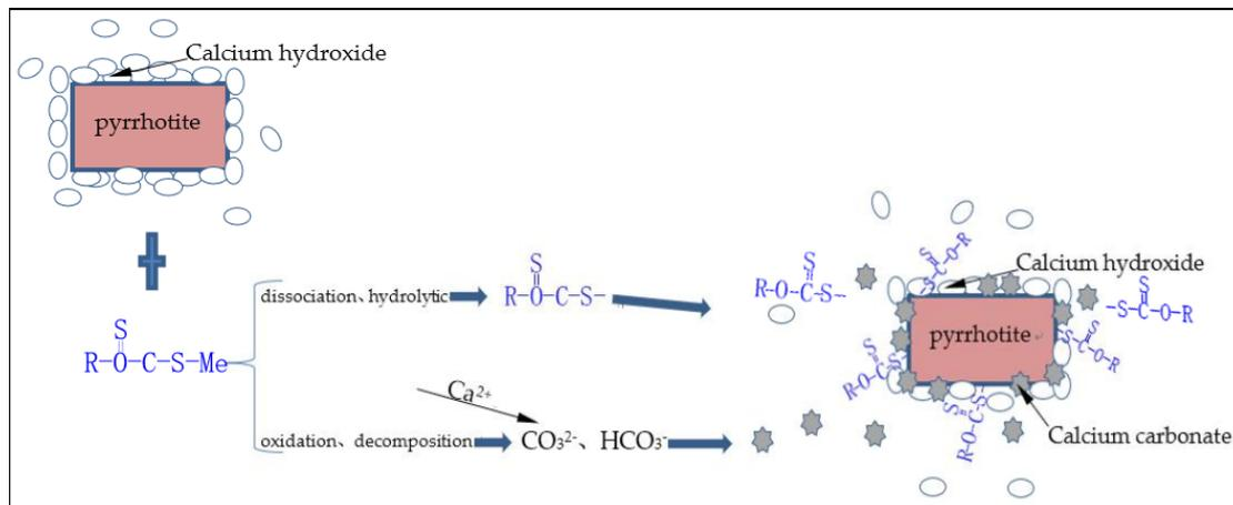
Fig. 8. The reaction process between pyrrhotite and collector
