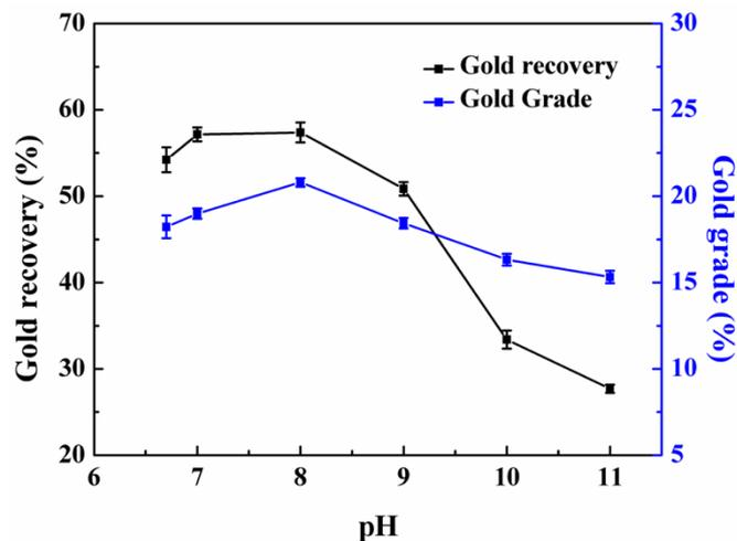
Fig. 3. Effects of pH on flotation index
