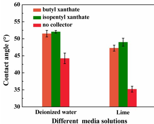
Fig. 5. Measurement of contact angle different medium solutions
