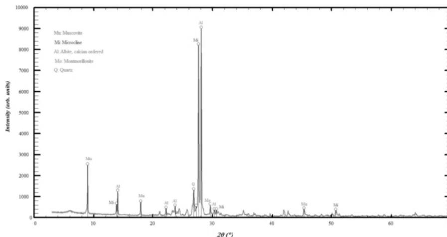
Fig. 1. Mineralogical analysis of nepheline syenite sample
