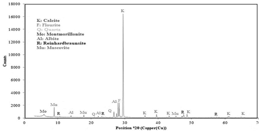
Fig. 7. XRD results of floated mineral in the conditions of 500 g/Mg DER NA7 at natural pH
