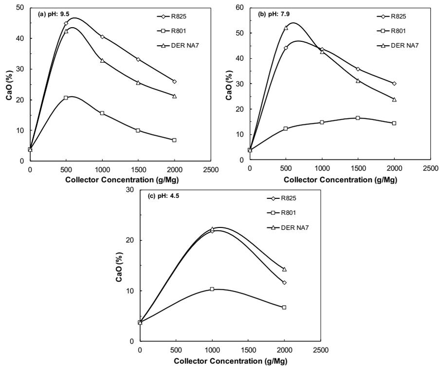
Fig. 6. CaO% change for collector types and amounts at different pH values (a) pH: 9.5 (basic), (b) 7.9 (natural), (c) 4.5 (acidic)
