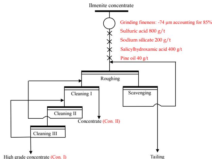
Fig. 3. Closed-circuit flotation flowsheet of ilmenite rough concentrate
