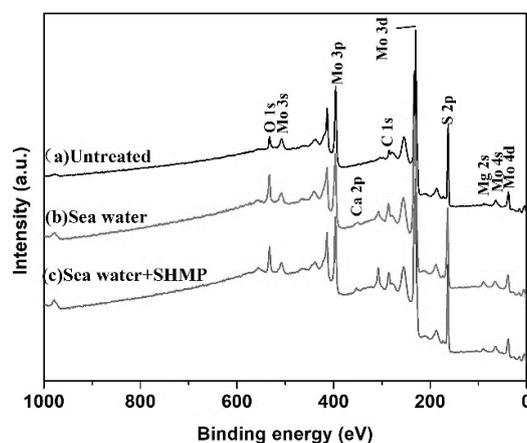
Fig. 5. XPS survey of  $\text{MoS}_2$ , (a) untreated, treated in (b) sea water and (c) sea water +SHMP at pH 10
