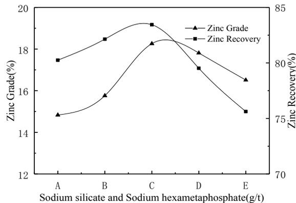
Fig. 4. The influence of  $\text{Na}_2\text{SiO}_3$  and  $(\text{NaPO}_3)_6$  dosage on Zn rougher flotation
