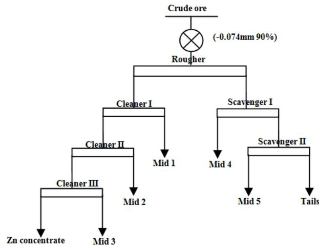
Fig. 7. Flow-sheets of open circuit test
