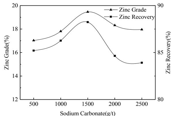
Fig. 3. The influence of  $\text{Na}_2\text{CO}_3$  dosage on Zn rougher flotation
