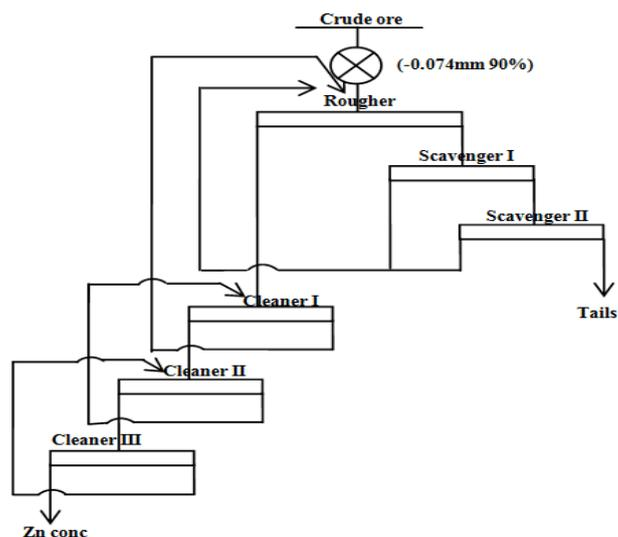
Fig. 8. Flow-sheets of closed-circuit tests
