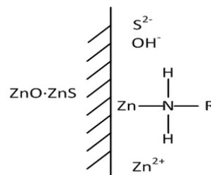
Fig. 1. The reaction between amine and zinc oxide minerals in the alkaline pulp
