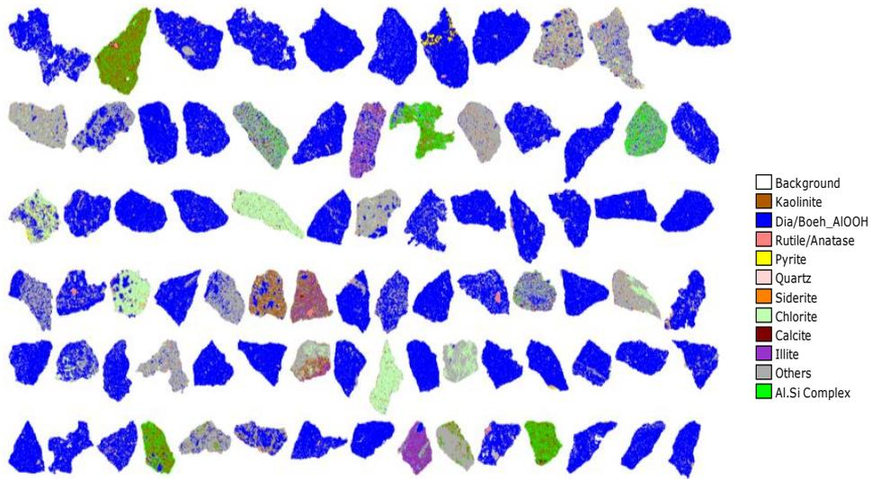
Fig. 1-1. +100 mesh mineral size scanning
