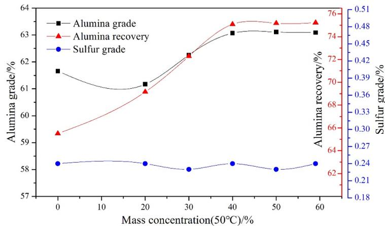
Fig. 3. Effect of mass concentration (50°C) on desulfurization and desilication towards concentrate indexes through synchronous flotation
