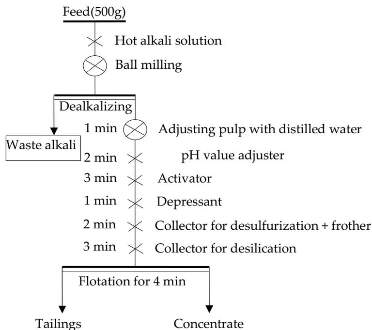
Fig. 2. Flotation flowsheet of the test samples
