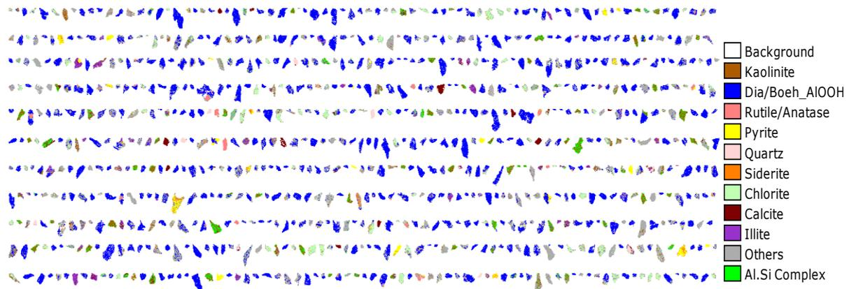
Fig. 1-4. +600 mesh mineral size scanning
