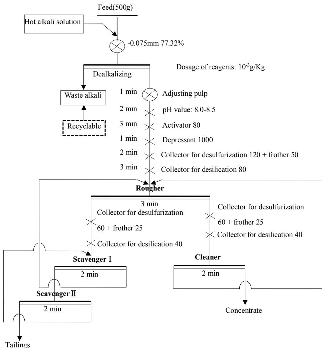
Fig. 5. Closed-circuit flotation flowsheet on desulfurization and desilication with a new process of surface pretreatment
