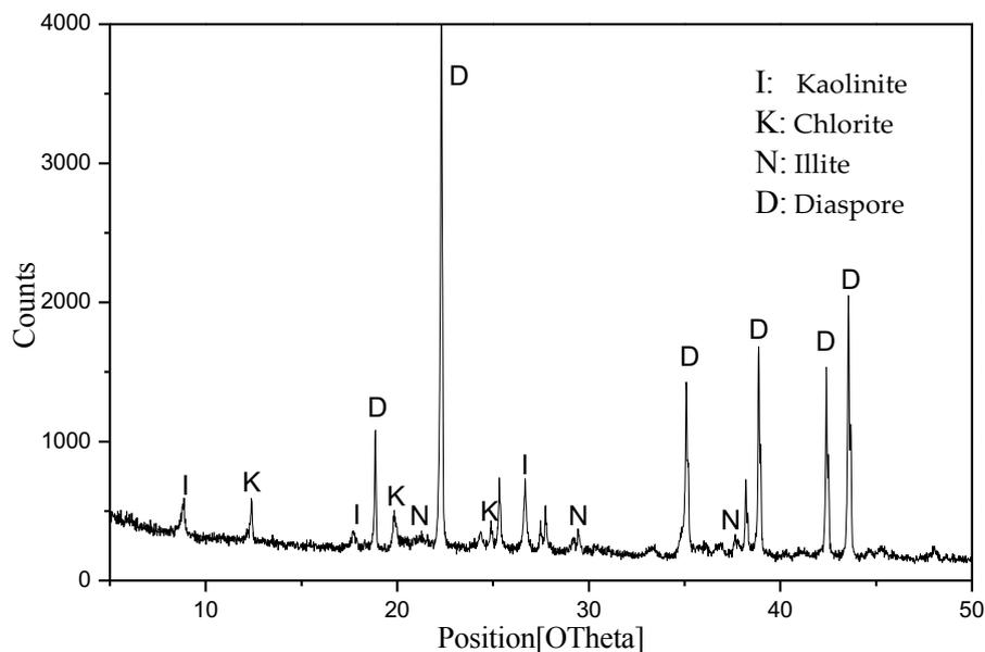
Fig. 6-1. XRD analysis of coarse particles with the distilled water pretreatment
