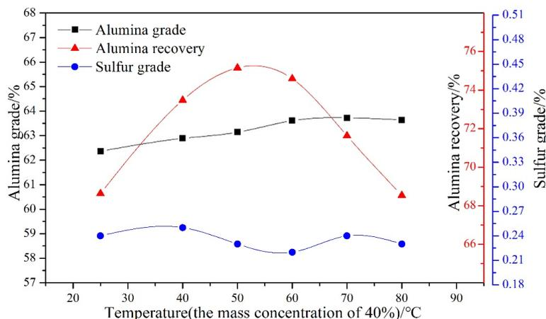
Fig. 4. Effect of hot alkali solution temperature (40% mass concentration) on desulfurization and desilication towards concentrate indexes through synchronous flotation
