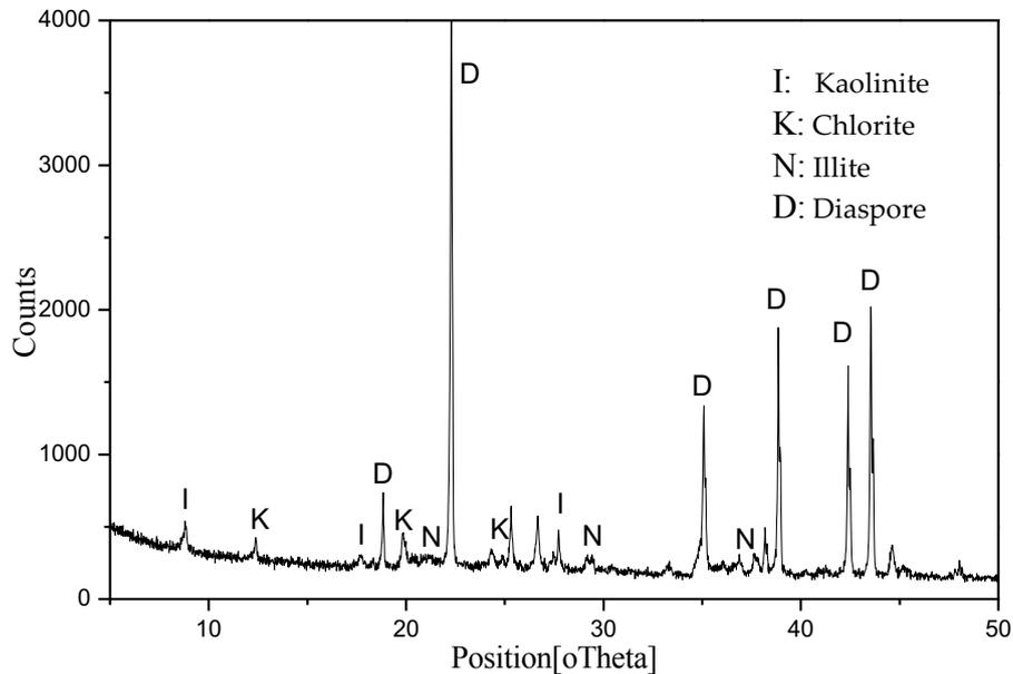
Fig. 6-2. XRD analysis of coarse particles with surface pretreatment
