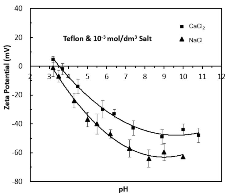
Fig. 4. Zeta potential-pH profiles of Teflon at  $1.10^{-3}$  mol/dm<sup>3</sup>  $\text{CaCl}_2$  and NaCl solutions
