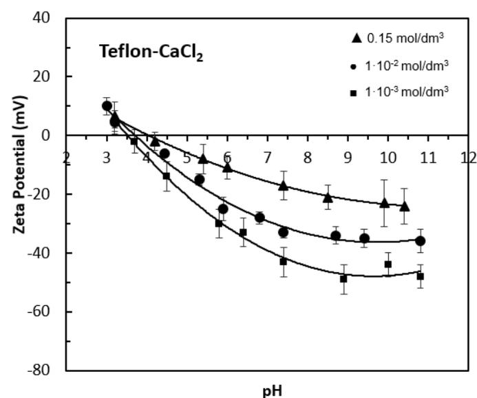
Fig. 3. Zeta potential-pH profiles of Teflon as a function of CaCl<sub>2</sub> concentration ( $1.10^{-3}$  mol/dm<sup>3</sup>,  $1.10^{-2}$  mol/dm<sup>3</sup>, and 0.15 mol/dm<sup>3</sup>)
