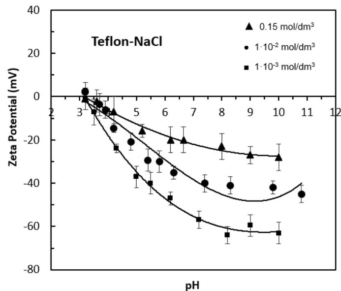
Fig. 2. Zeta potential-pH profiles of Teflon as a function of NaCl concentration ( $1.10^{-3}$  mol/dm<sup>3</sup>,  $1.10^{-2}$  mol/dm<sup>3</sup>, and 0.15 mol/dm<sup>3</sup>)
