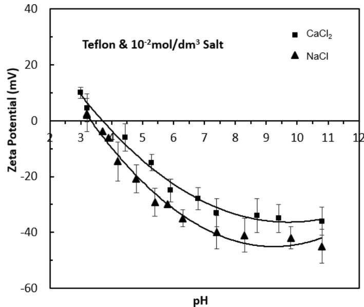
Fig. 5. Zeta potential-pH profiles of Teflon at  $1.10^{-2}$  mol/dm<sup>3</sup> CaCl<sub>2</sub> and NaCl solutions
