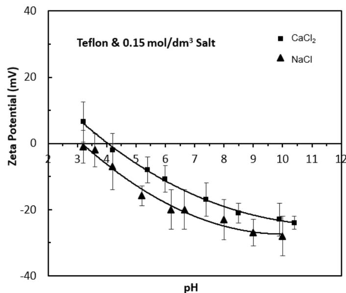
Fig. 6. Zeta potential-pH profiles of Teflon at 0.15 mol/dm<sup>3</sup> CaCl<sub>2</sub> and NaCl solutions
