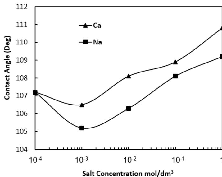
Fig. 7. Contact angles of the plate Teflon as a function of salt concentration
