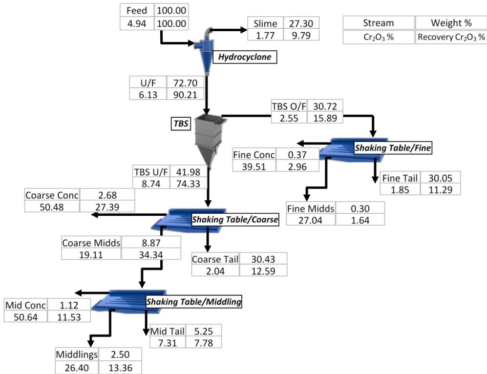
Fig. 5. Beneficiation test results of alternative 1 (TBS followed by shaking tables)
