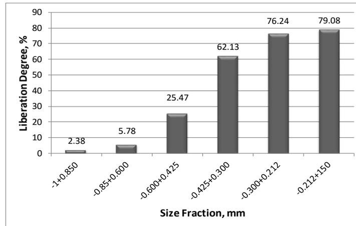
Fig. 3. Liberation degree of chromite at sizes less than 1 mm
