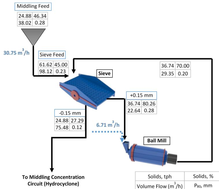
Fig. 7. Grinding circuit of middling products
