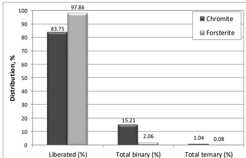
Fig. 2. Liberation and locking states of chromite and forsterite minerals
