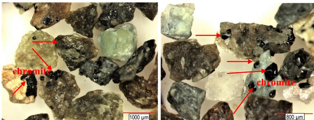
Fig. 4. Stereomicroscope images of chromite particles at  $-1$  mm size
