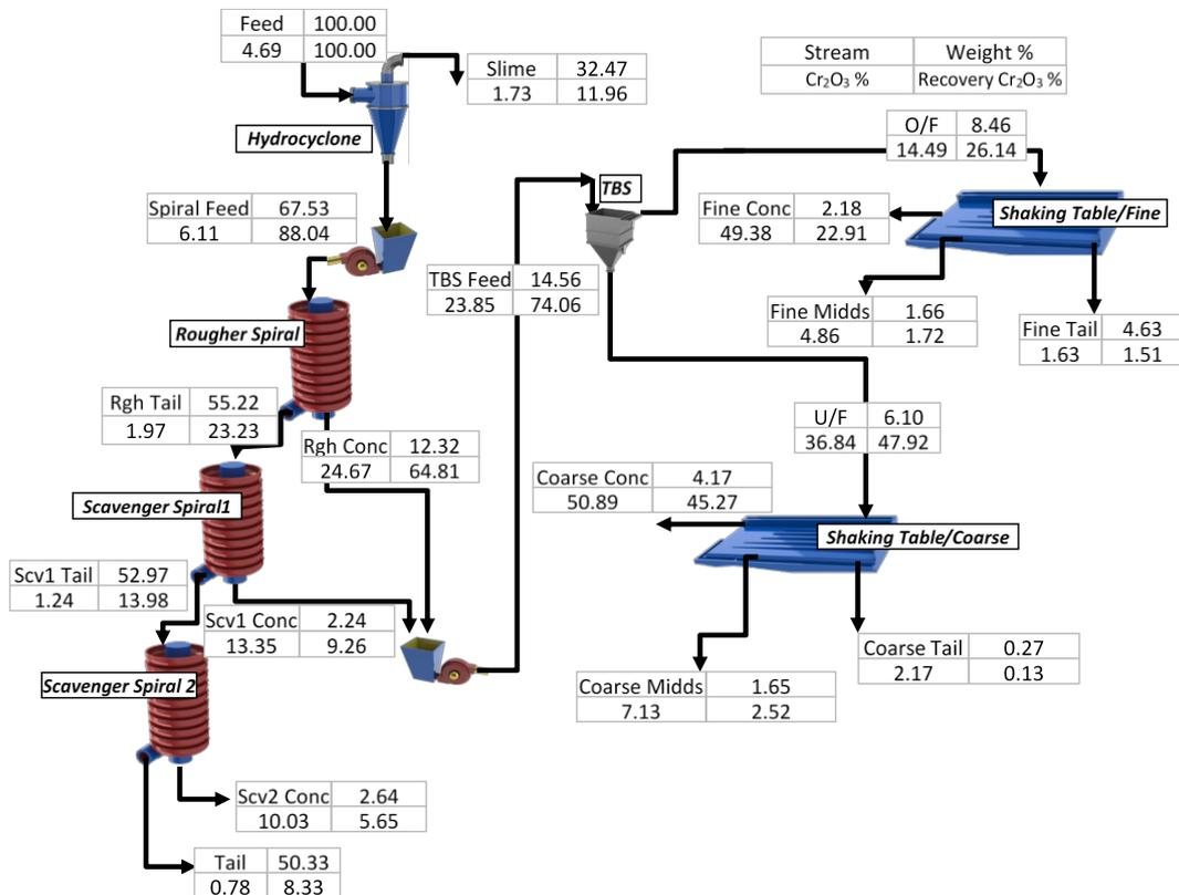
Fig. 6. Beneficiation test results of alternative 2 (spiral concentrator, TBS, and shaking tables) open circuit
