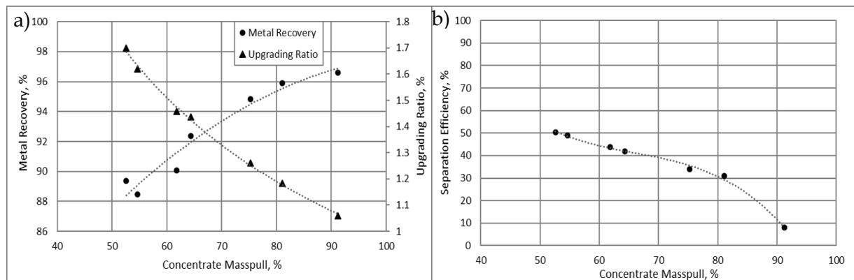
Fig. 10. Metallurgical performance summary (a) and separation efficiency values (b) of plant trials
