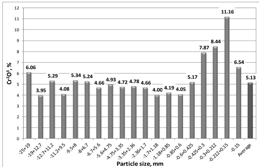
Fig. 1. Size-by-assay analysis of ROM chromium ore
