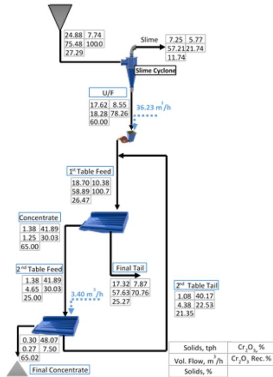
Fig. 8. Concentration circuit of middling products and their mass balance
