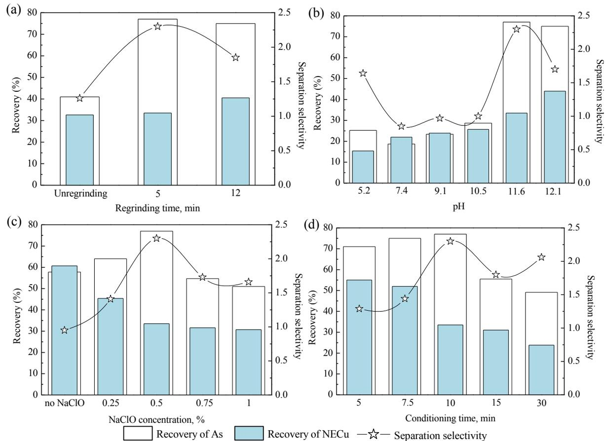
Fig. 8. The effect regrinding (a), pH (b), NaClO concentration (c), conditioning time (d) on separation of enargite from NECu minerals
