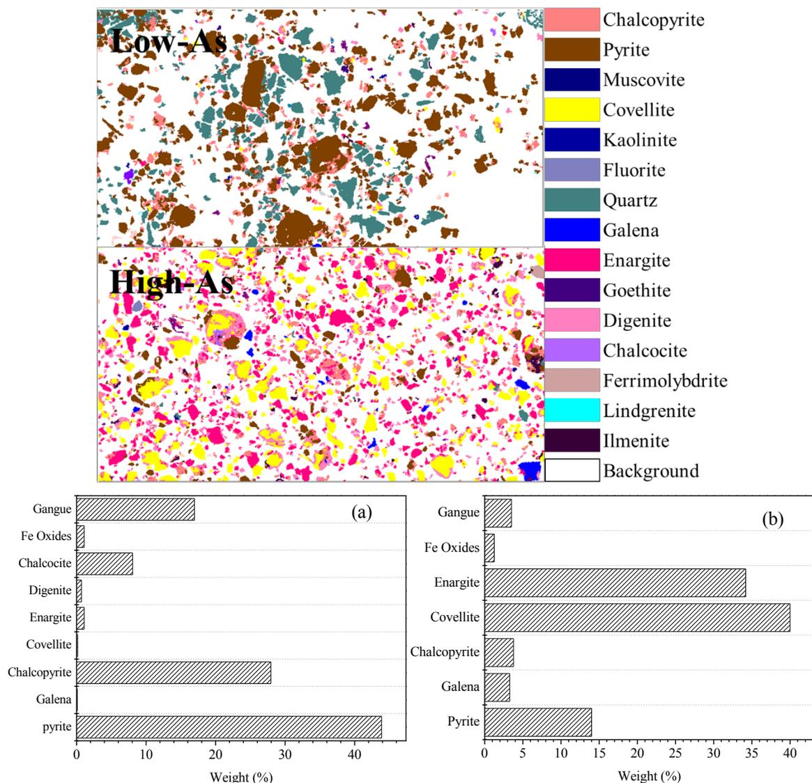
Fig. 12. The MLA images and minerals weight distribution of the final low-As (a) and high-As (b) copper concentrates
