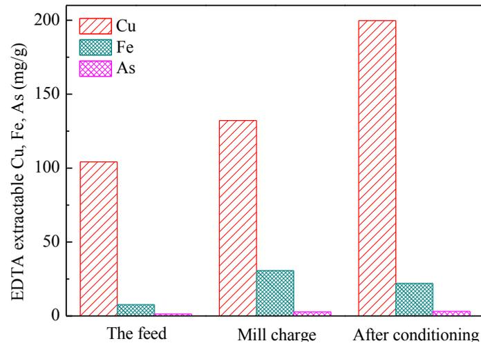
Fig. 10. EDTA extraction results from different treatment stages
