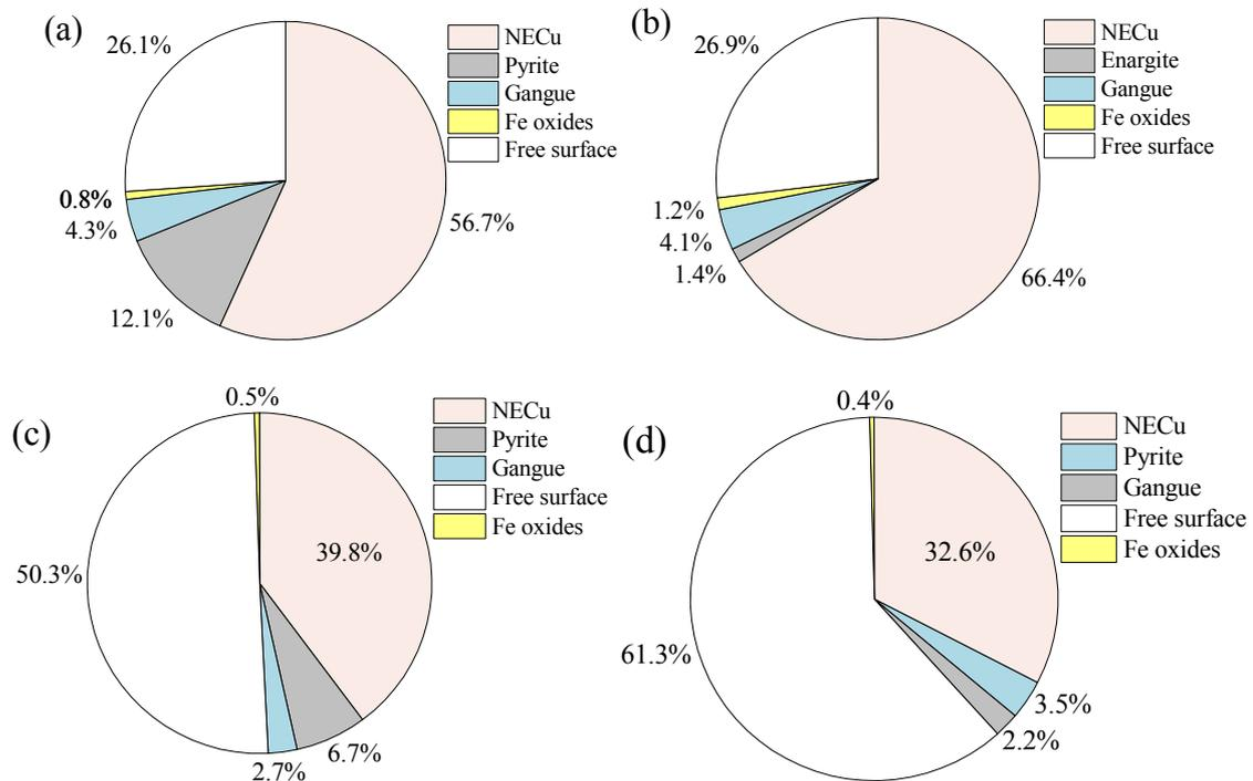
Fig. 7. Mineral association for enargite in the copper concentrate(a) and regrinding products(regrinding 5min (c), 12 min (d)), and for pyrite (b) in the copper concentrate
