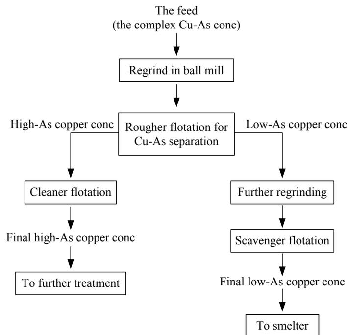
Fig. 11. Proposed conceptual flowsheet for separation enargite from NECu minerals
