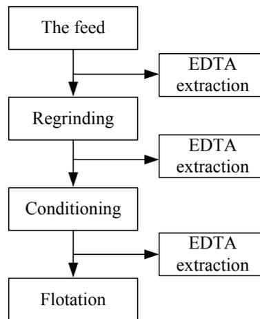
Fig. 3. The flowchart of EDTA extraction tests
