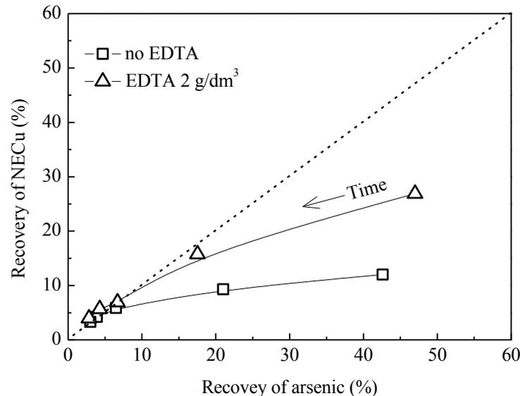
Fig. 9. Flotation recovery of arsenic and NECu as a function of flotation time. Flotation conditions: regrinding 5 min, pH 11.6, 0.5% (v/v) NaClO and conditioning time 10 min
