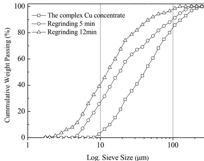
Fig. 2. Particle size distributions of the complex copper concentrate and regrinding products
