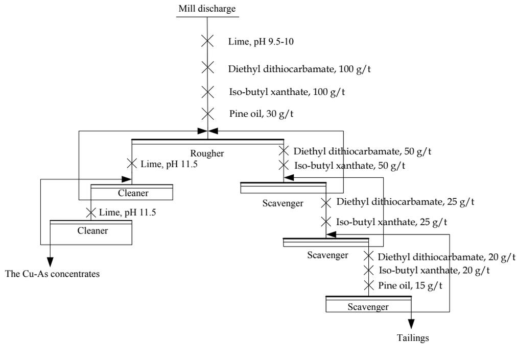
Fig. 1. The flotation flowsheet of the copper flotation plant
