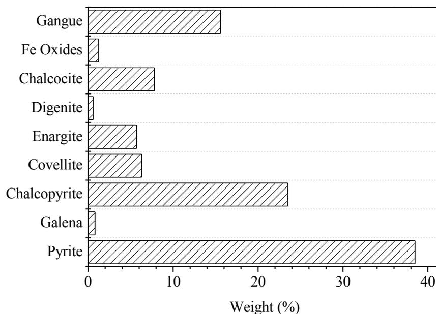
Fig. 5. The minerals weight distribution of the copper concentrate
